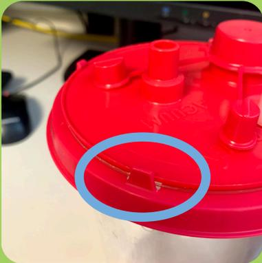
4. Place lid on top of disposable cannister and snap firmly into place. Be sure to snap connections around entire circumference of cannister.
